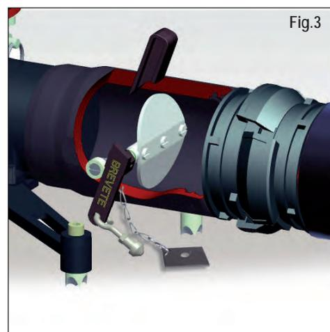
**⚠ CHECK BEFORE ANY OPERATION THAT NOTHING PREVENTS THE GOOD OPERATING OF THE VSC (swinging of the lever on its axis and free oscillation of the release).**
